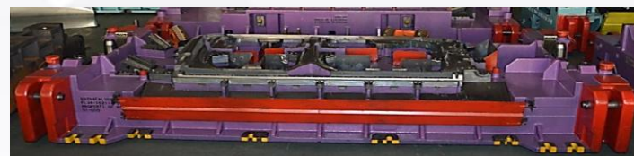
Stamping die exported to Ford America for F-150 (Aluminum Part Material)
